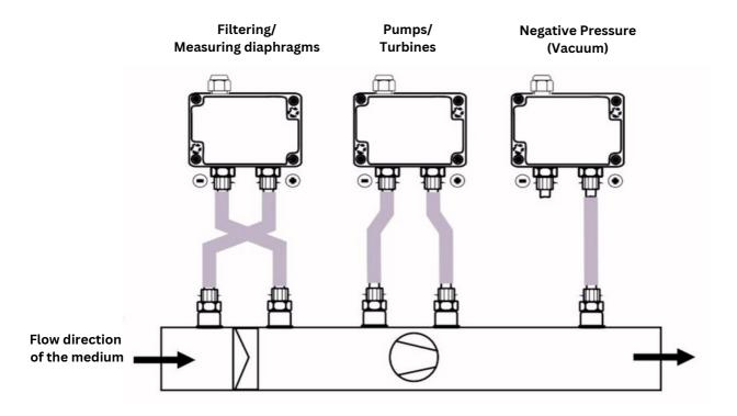
Depending on the medium and static pressure range, tubing or pipework systems are used for the process connection.
